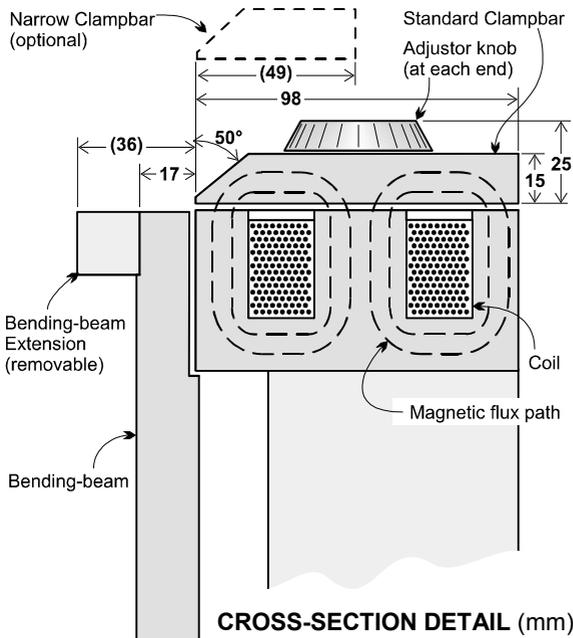
CROSS-SECTION DETAIL (mm)
