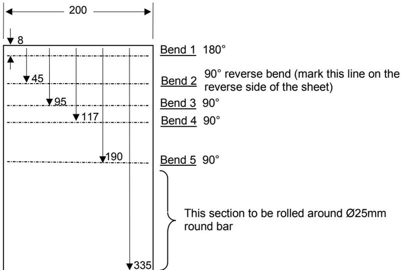
3. Align **Bend 1** and form a lip on the edge of the workpiece. (See "FOLDED LIP")
