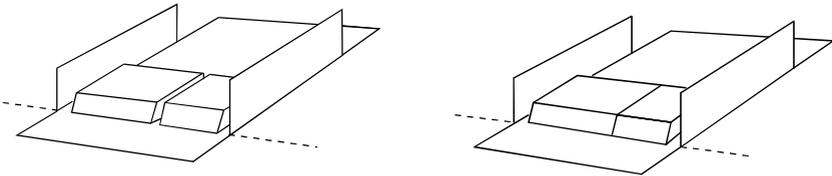
For bends up to 70 mm long, just select the largest clamp piece that will fit. For longer lengths it may be necessary to use several clamp pieces. Just select the longest clampbar that will fit in, then the longest that will fit in the remaining gap, and possibly a third one, thus making up the required length.
